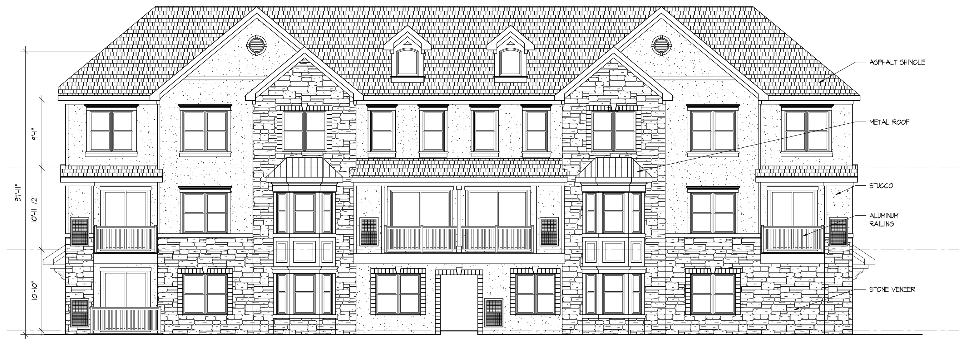
BUILDING A - FRONT ELEVATION
